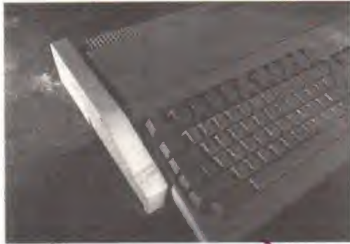
Although the SupraRAM has few components of its own, adding 4Mb of RAM could necessitate buying a bigger power supply.
